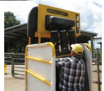
23. Repeat this procedure on the vacuum duct and bezel. Make sure the flex duct tube is vertical and the nozzle top edge is level. Instead of screws that tap into the plastic as on the pressure duct, this vacuum duct uses machine screws and locking nuts so you must run a drill thru the holds in the duct and thru the vinyl. When all screws are secured cut out the vinyl using a sharp blade with the inside of the nozzle as a guide.
