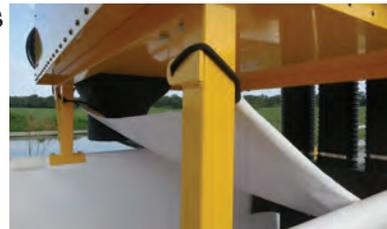
25. Intall the collection bag on the ring below the collection chamber with the hose clamp. Add the plastic closure clamp to the bottom of the collection bag.
