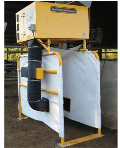
18. Install the 6" flex duct on the vacuum nozzle and tighten the clamp. Install this assembly onto vacuum manifold on the right side of unit with the pressure nozzle bezel parallel with the rails and tighten top clamp. The insides of this vacuum duct should also be approximately 24" from the ground.
