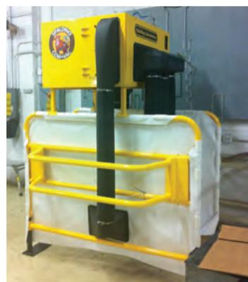
28. Plug the power cord into a 20amp 120 volt dedicated circuit with a GFI breaker. Turn the unit on. The CowVac should pull approximatly 15 amps when running, maximum 16 amps. This is pre-set at the factory but can be adjusted in the field by adjusting the variable pully on the motor. Please call if you need to do this.
