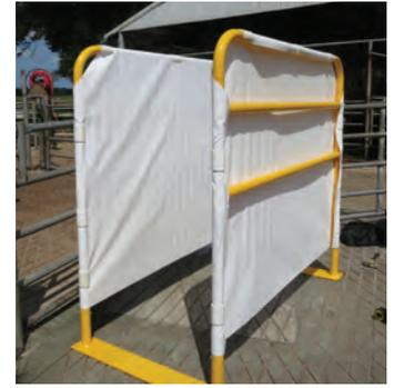
12. If your unit does not have the large cutouts for the ducts these curtains are interchangeable. You should center the curtains on the side rails with the cut corner at the top. Wrap the curtain about 3/4 of the way around the top rails. You will later cut out the large duct holes after mounting the ducts to the curtains.
