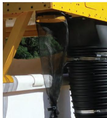
26. Install the “Nerf Bars” that protect the flex ducts if your cows will have access to the side of the CowVac. These bolt on with 2 3/4” bolts and nuts. Add bungee cords to each of the vacum ducts to pull them inward. Secure bungee to the horizontal rail with 2 bolts and large fender washers.
