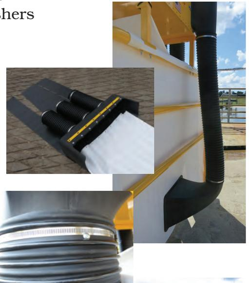
21. Once all ducts are secured and in position with clamps install 2 SS screws & fender washers thru the flex duct into molded manifold parts to provide additional retention. Without these screws the ducts could slide off.
