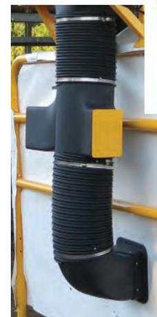
17. Install the pressure duct assembly over black plastic fitting on bottom of the left side of the CowVac unit (below the power switch). The pressure nozzle bezel should be parallel with the rails. When installed the top of the inside of the bottom duct should be approximately 24" from the ground with the vertical rails in the middle position.
