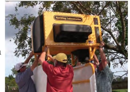
14. Mount the CowVac unit on the top rails by lifting it with a person on each corner. The heaviest corner is the one with the power switch so put your burliest guy there. Set unit over mounting holes in top rail using a 5/16"x 2 3/4" bolt to align the holes on curtain & top rail with the holes in the half round mounting feet. Secure with 8 - 5/16"x 2 3/4" hex bolts & lock nuts to top rails.
